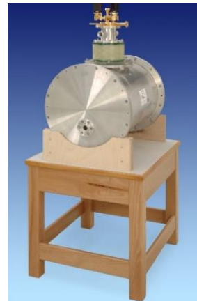
Figure 1: OPM (left) inside a 40 cm long shielding and SQUID (right) based magnetorelaxometry device for characterization of magnetic nanoparticles.
