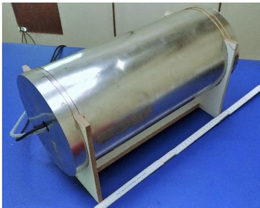
Figure 1: OPM (left) inside a 40 cm long shielding and SQUID (right) based magnetorelaxometry device for characterization of magnetic nanoparticles.
