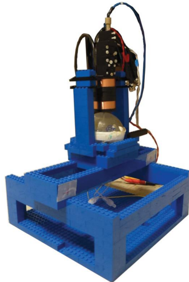
Figure 1. OPM measurements of a phantom. The sensor is mounted on top using LEGO bricks.
