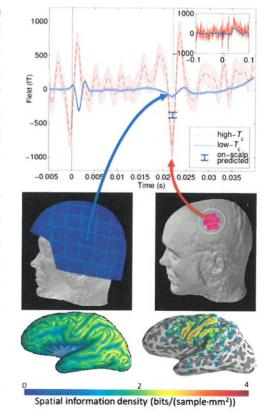
Experimental (top) and theoretical (bottom) demonstrations of the advantages of high- $T_c$  SQUID-based on-scalp MEG (adapted from [2,3]).
